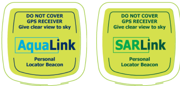
Figure 4 – GPS Receiver Location
